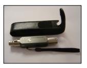
Each of these functions is activated by pressing the mode button (labelled ON). Press the ON button to cycle through each of the functions in turn. From the powered off state, press the ON button once to activate the Torch function.
