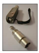
It is possible to test installed cabling using the Cable Test, by combining two devices. Place one of each of the devices on the end of the cable (you will require a female-female jumper on one of the ends) and place both Cable Tests in Cable Test mode. The test will now occur throughout the cable, and indicate any problems in the installed cabling.
