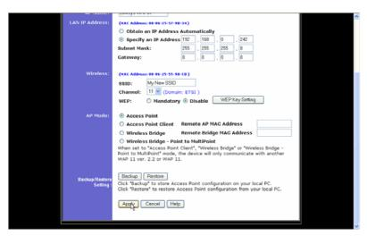
A final note on changing the channels. Although channels 1 and 2 are numerically different the physical frequencies which they represent overlap. Depending on which other wireless networks are in use in the local area, you may need to reconfigure the units to respond to different channels.
