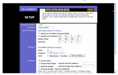
Here it can be seen that this WAP has its SSID set to A and its Channel is set to 1. If the SSID of the boxes are also set to A then the system will work and the encoder box will route its airborne DMX data via the WAP, if there is any discrepancy it will not work. Please note the SSID is Case Sensitive.
