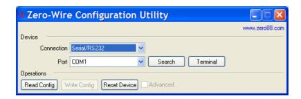
Select the COM port which the Zero Wire box has been connected to, or press Search.
