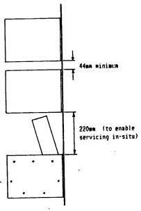
The sides of the Rackmaster may be removed, changed over (left for right and right for left) and replaced so that the mounting flanges are at the rear.
