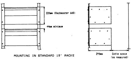
For easier servicing, mount each Rackmaster on a standard telescopic rack slide.
