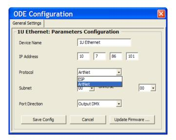
11. Assign your 1 Universe Ethernet Box to a Subnet and Universe in the Art-Net range of possible locations. If you only have one 1 Universe Ethernet Box, the default of 0,0 may be suitable, but when multiple devices are used then take care as to which you assign where, and consider labeling the outside of the box, perhaps with tape and a permanent marker, or by using a plastic stick-on label, so that you can deploy and troubleshoot it easily.
