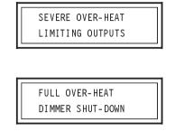
Normal operation will resume as soon as the internal temperature of the dimmer has reduced.
