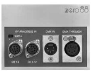
to 512 channels, any 12 ( or 6 on the ID 625 ) of which may be selected to control the dimmer.
